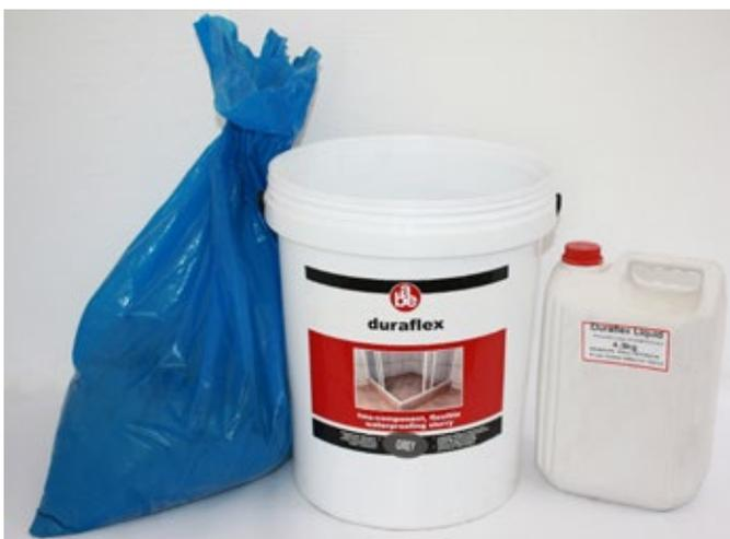
Apply a second coat and third coat of **dura.@flex** to the whole area to be waterproofed. Apply coats at right angles to each other, allowing 16 hours between coats. **dura.@flex** should not be applied thicker than 1kg per coat per m2.
