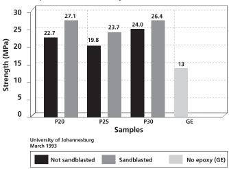
Compressive strength of specimens bonded with **epidermix 116** using mortar of different strengths. Mortar surfaces are either sandblasted or not sandblasted prior to application of **epidermix 116**. GE is control sample with no **epidermix 116**.
