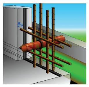
Joint surface must be clean and dry and any protrusions greater than 3mm high ground or chipped off.
