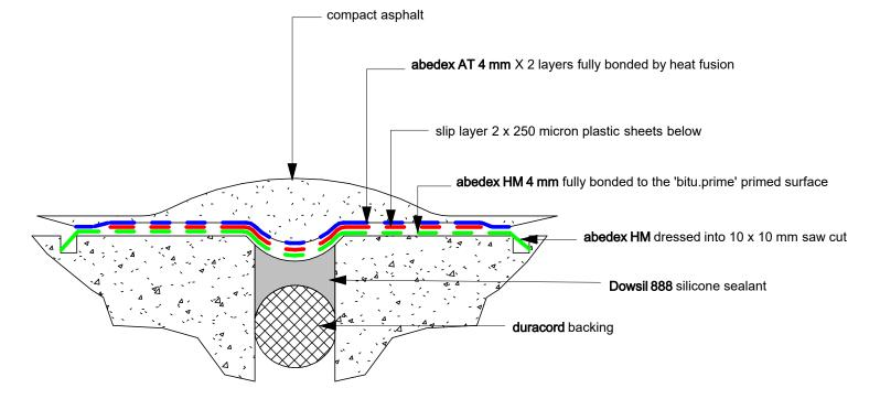
Note: abedex HM fully bonded a minimum 250 mm either side of the joint The plastic slip layer to bridge the joint by 250 mm either side of the joint
