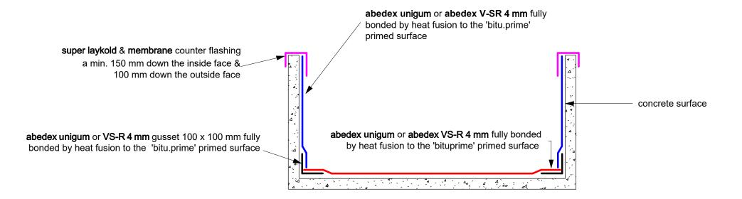
Note: Clean by high pressure water cleaning the entire surface to remove all curing compound, dirt, fungal growth etc. and allow to dry. All unsound material to be removed and repaired prior to waterproofing.
