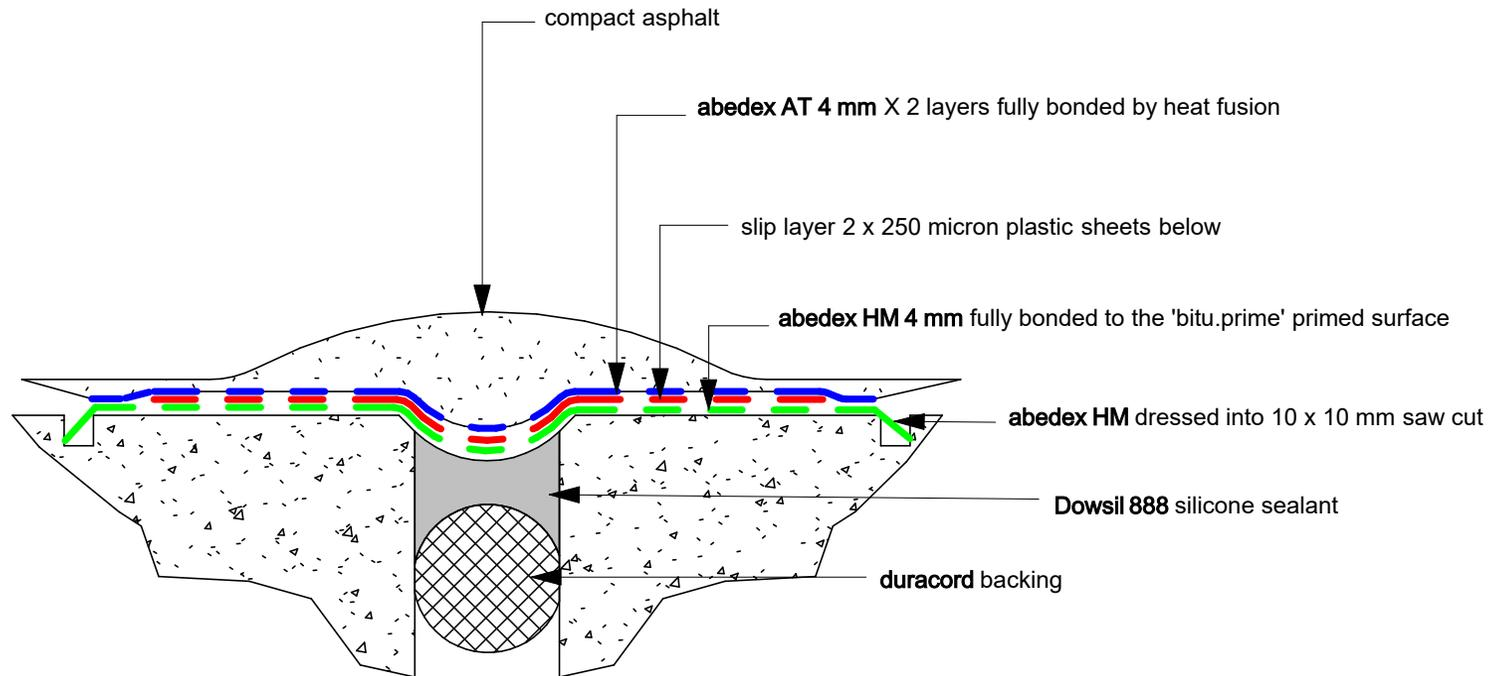
**Note: abedex HM fully bonded a minimum 250 mm either side of the joint**
